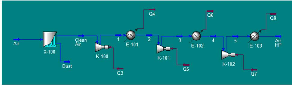
Figure 6. Air Pre-Treatment Process
