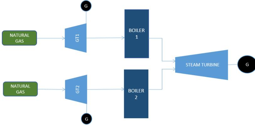
Figure 3.3: Illustration of plant topology, CCGT [29]
