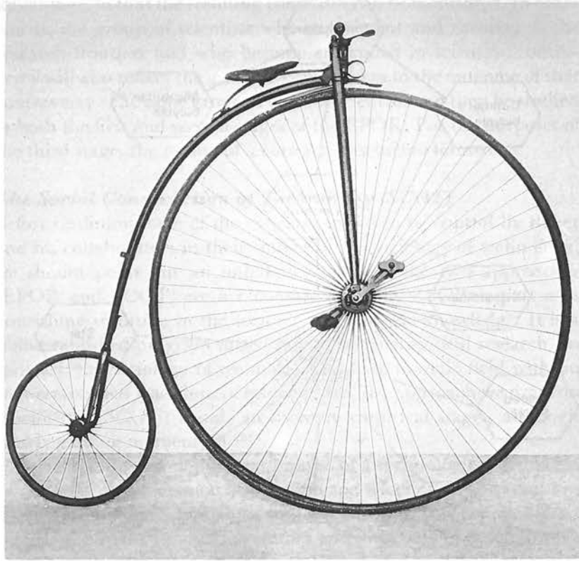
Figure 3 A typical Penny Farthing, the Bayliss-Thomson Ordinary (1878). Photograph courtesy of the Trustees of the Science Museum, London.
