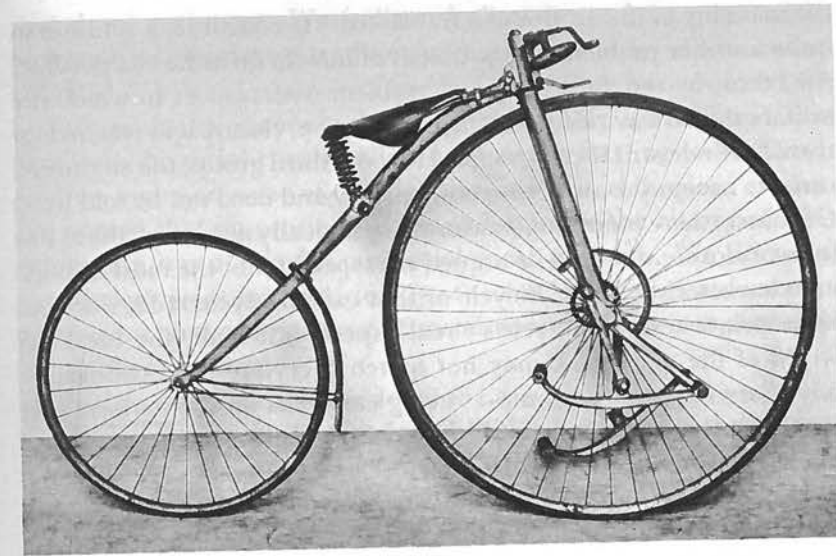
Figure 16 Geared Facile bicycle (1888). Photograph courtesy of the Trustees of the Science Museum, London.
