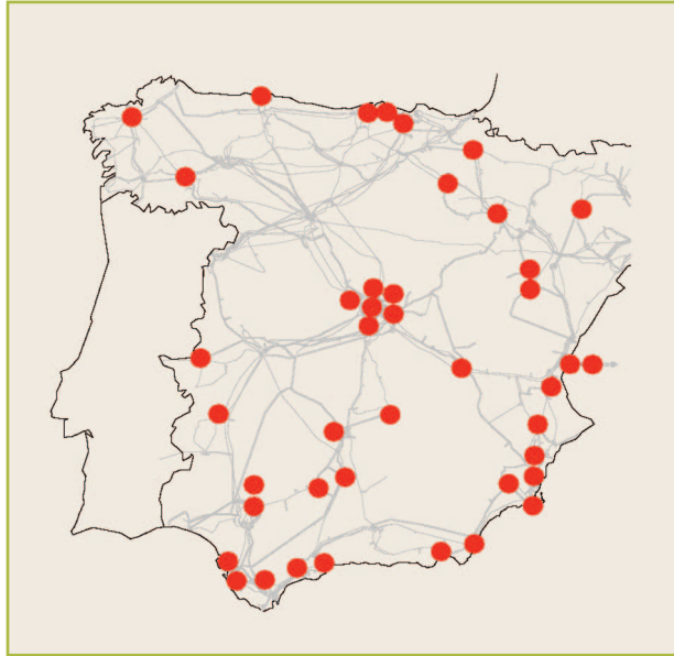
figure 9. Expansion plan for 2005–2011: new 400/220-kV transformers.
